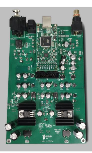
The DAC reads files with conversion up to 784 Khz in PCM and DSD 256 in Dop or DSD 1024 natively.
