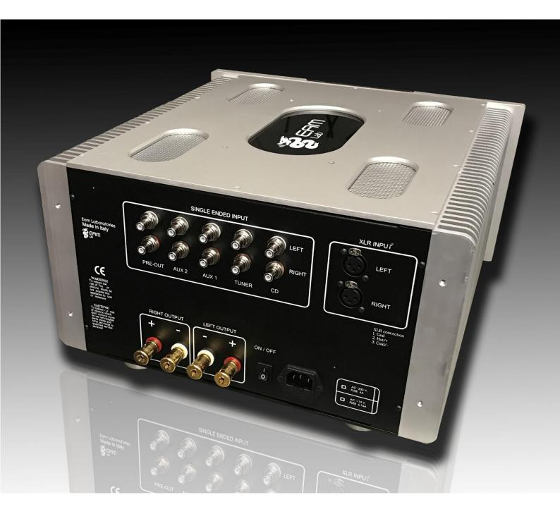
WBT rhodium-plated connectors for the best possible connection between sources and loudspeakers
