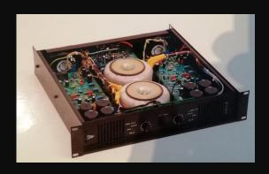
During 2001 the PA2600 was produced together with its smaller brothers, the PA2400 and PA2200. very compact amplifier capable of over 500Wrms per channel at 8 ohm. Widely used with great satisfaction on tours due to its lightness (for the time), reliability and transportability.
